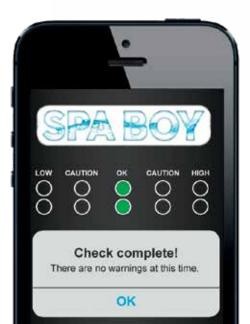
A **medical grade sensor** measures ORP and pH for water quality. The **SpaBoy controller** analyzes the data and activates the **electrolytic cell** when the water quality drops below the set point. The **EcoPack** control system integrates SpaBoy with the main hot tub controls and enables 2 way communication with the Arctic Spas App or myarcticspa.com via the internet.
